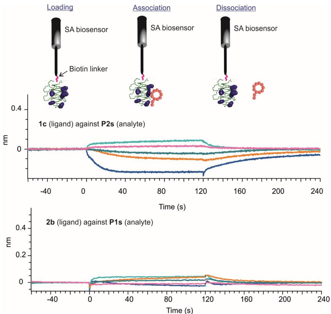
**Figure S5.** BLI control experiments to confirm the selective and specific binding of each teMP **3a** and **4a** to their corresponding foldamer sequence **1c** and **2b** respectively. For each experiment, five concentrations of peptide were used, ranging from 39-2.5  $\mu\text{M}$  for **3a** and **4a**. In both assays, a double referencing was performed to remove any nonspecific binding of the peptide macrocycle to the SA-surface.
