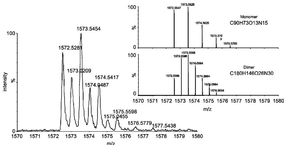
**Figure 4.** Experimental high-resolution ESI mass spectrum of **2** showing the isotopic mass distribution of the single helical monomer  $[\text{M}+\text{H}]^+$ , which adds to that of the diprotonated double helical dimer  $[2\text{M}+2\text{H}]^{2+}$ . The inset shows the theoretical isotopic distributions of  $[\text{M}+\text{H}]^+$  (top) and  $[2\text{M}+2\text{H}]^{2+}$  (bottom).
